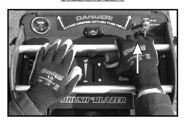
Keep your left hand on the left steering control handle. Push the right steering control handle forward to steer to the left. Push the right steering control slightly to steer slowly. Pushing the control harder will execute a sharper turn.
